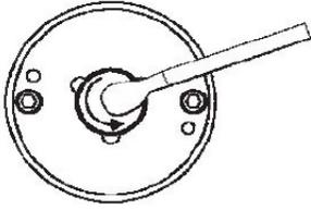
**Note:** If your system is equipped with Air Assist, you must remove the beam window protector to gain access to this optic to clean it. Rotate the beam window protector counterclockwise and then off at a 45-degree angle. If the beam window protector is stuck, use a 1/16 Allen wrench to slightly loosen the screw and try again. Set the protector off to the side and clean the optic, if necessary. Reinstall the beam window protector being careful not to scratch the optic.
