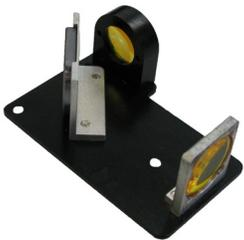
First, never clean the optics if they appear to be clean. Excessive cleaning will prematurely remove the optical coating. Also, try not to touch the optical surface as the oils on your skin may damage the coating. Finally, never clean the optics right after they have been used to process material or immediately after cleaning, since thermal shock can cause the optics to crack.
